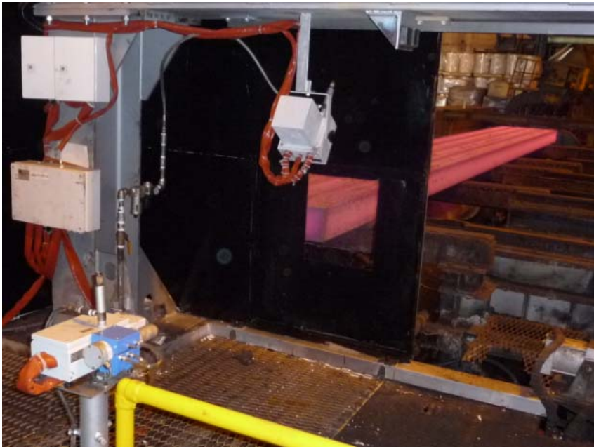
Fig.1: Camera installation at bloom marking machines, camera with cooling and laser trigger in the foreground
